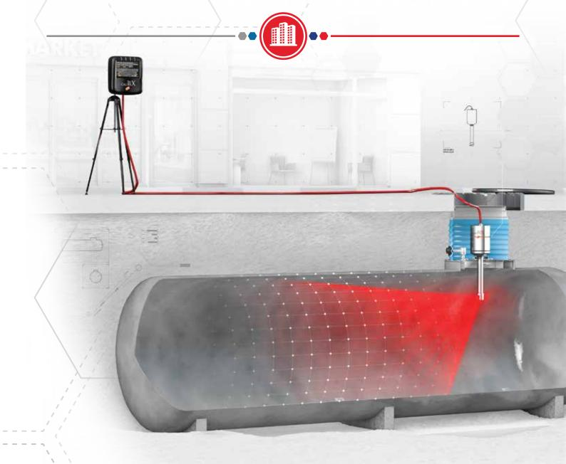
Safely calibrating fuel tanks with high accuracy, even with fuel inside, in 30 min.
